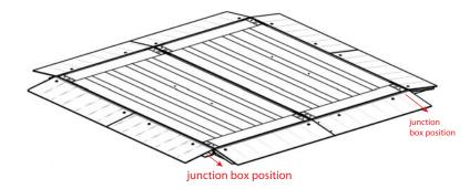
(10) Assembly four small ramps on four corners .
