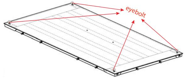
(3) Lift up platform by chains to install feet .
